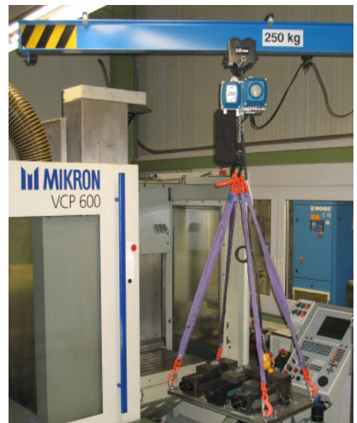
The crane for heavy work pieces or pre-equipped clamping systems
