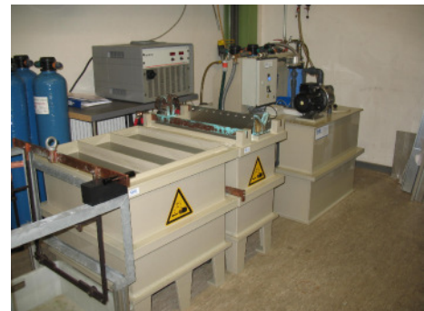
Degreasing machine for preparation of subassemblies to soldering and welding
